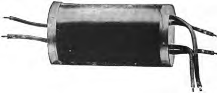
FIG. 334.—A Typical Jump-Spark Circuit Induction Coil—the “American” Double Terminal Coil. This coil, which is one of the most effective in use, has a double wound secondary with sparking contacts for two jump-spark plugs. According to the manufacturers, where two plugs are required to spark simultaneously, the best results are obtained by using a coil with two secondary windings and three secondary lead wires, one of which is grounded, and one carried to each of the plugs. The circuit thus formed gives, according to claims, the strongest possible effect in gas engine ignition.
